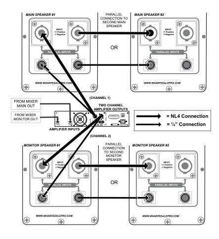
**NOTE**: This configuration represents a 4 ohm load to each output channel of the amplifier.
